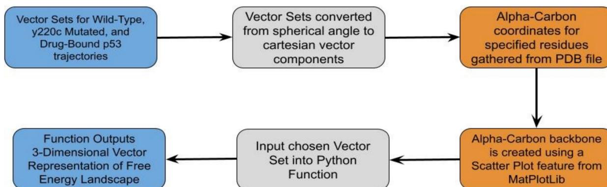
Figure 4: Flowchart Depicting Creation of 3-Dimensional Vector Representations using Matplotlib
