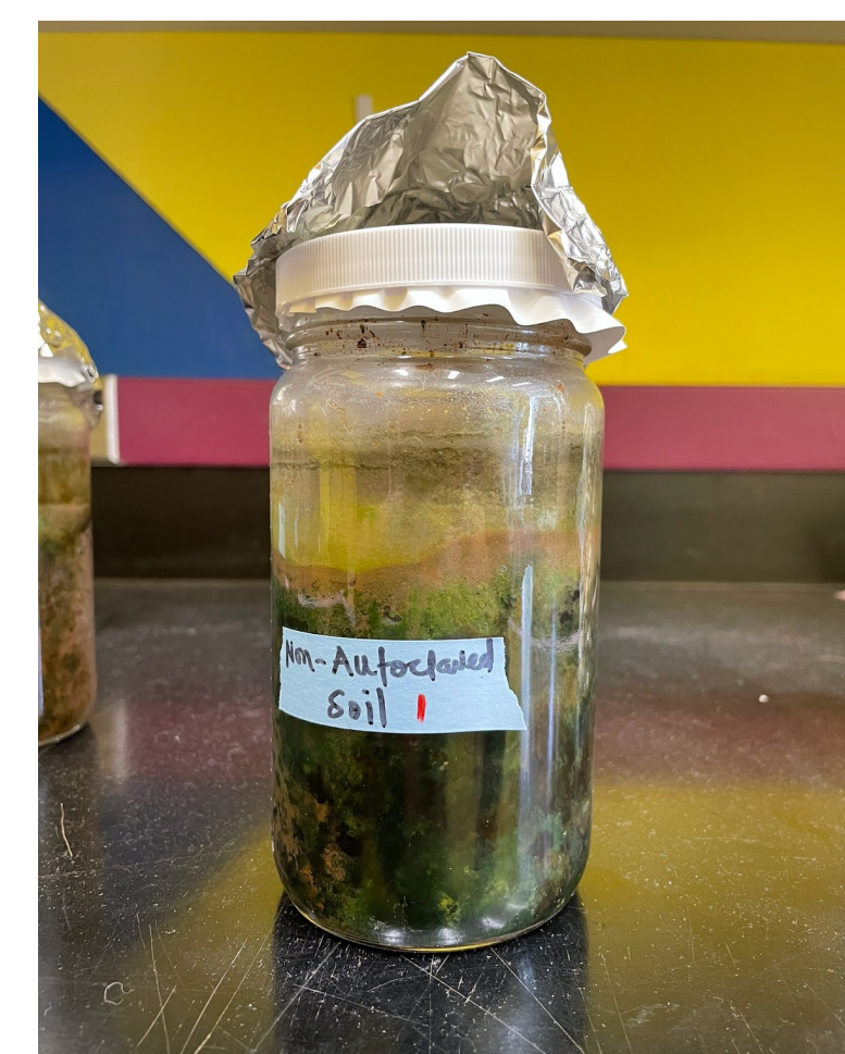
Figure 2: Winogradsky column used in experiment
